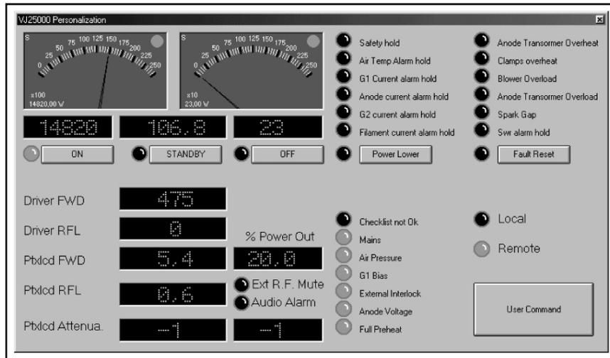
In order to change some levels such as attenuation of the inputs and the output power percentage of the PTXLCD, double click on the measurement that you wish to change and insert the new value required.
