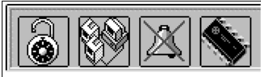
The password: The first icon represents the password. If this icon is activated in the station a closed lock appears on a yellow background, otherwise it is open as shown on the picture.
