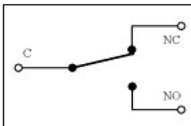
The maximum current that could be made flow through the contacts is of 500mA to 24V.
