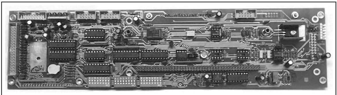
Includes a liquid crystal graphics display, the encoder and several LEDs. This card is not present in model TLC300.
