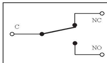
The maximum current which can be passed through the contacts is 500mA at 24V.
