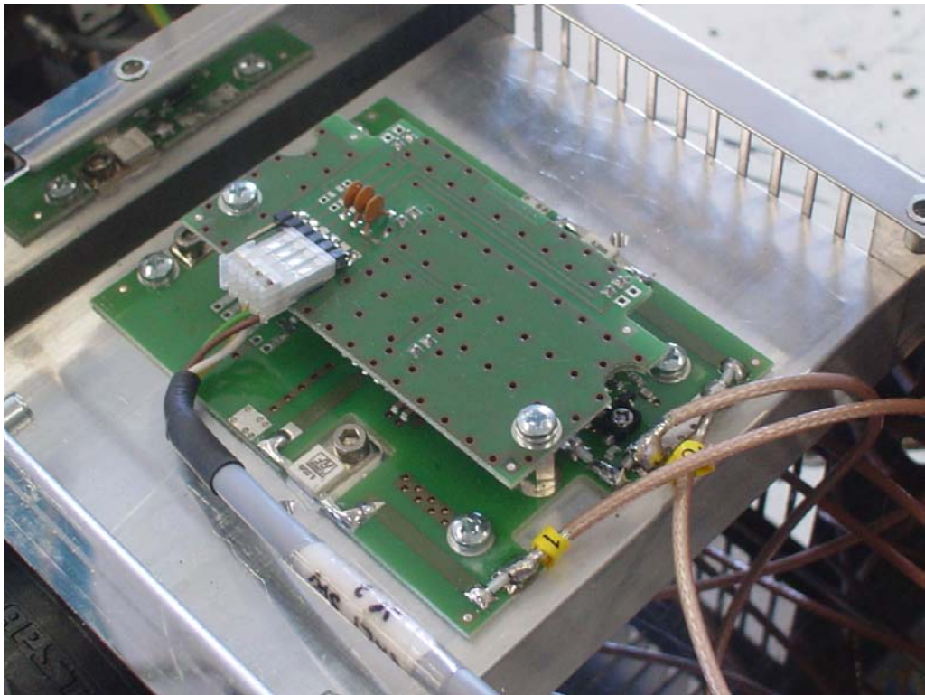
Exciter RF switch
