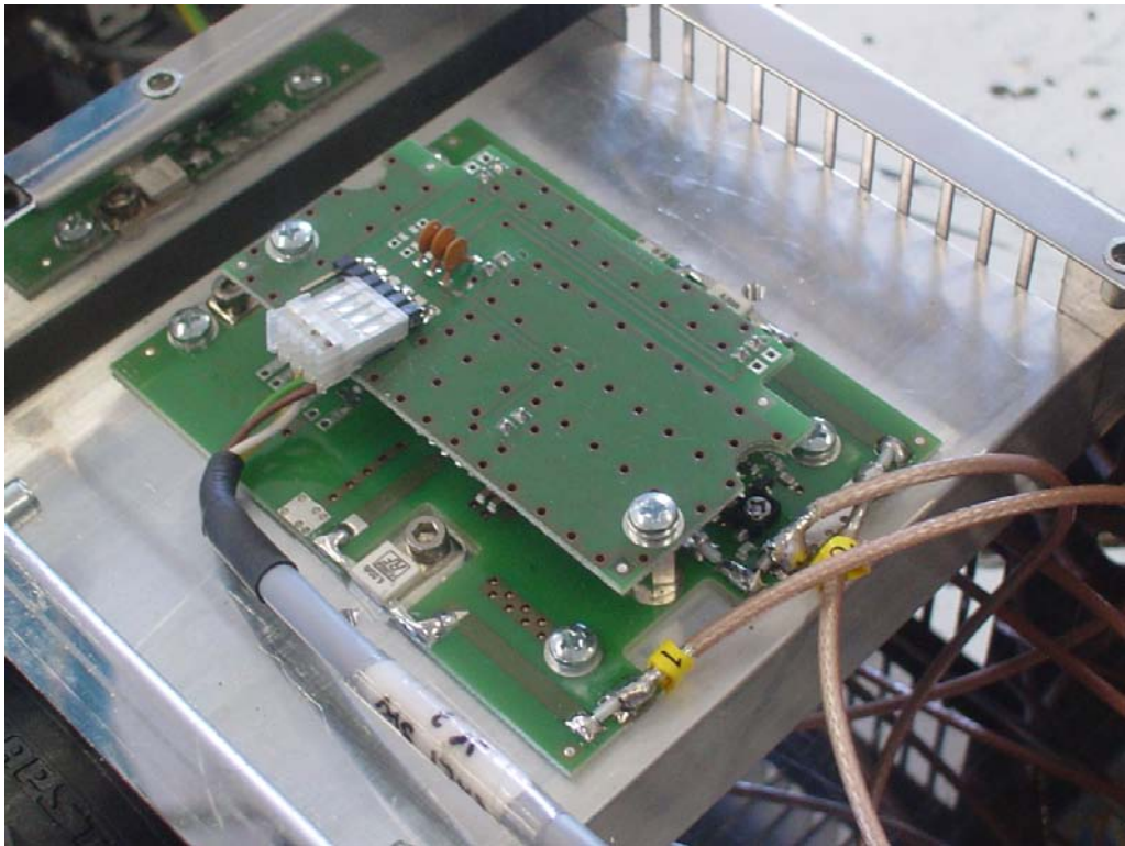
Exciter RF switch
