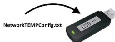
Edit NetworkTEMPConfig.txt and write inside the temporary IP you want set for your TRDS4002-LUXOR-D. The syntax has to be: **IP/24**
