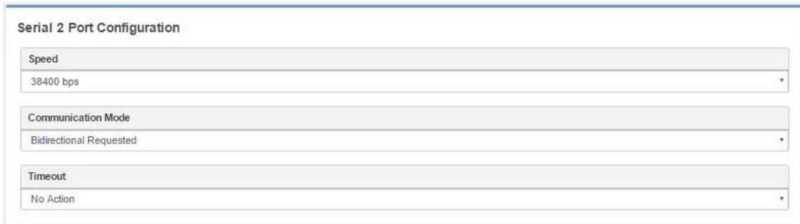
The screenshot shows a configuration window titled "Serial 2 Port Configuration". It contains three dropdown menus: "Speed" set to "38400 bps", "Communication Mode" set to "Bidirectional Requested", and "Timeout" set to "No Action".
