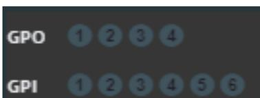
**GPO:** You can connect the device to a maximum of 4 GPO devices(GPO1, GPO2, GPO3, GPO4). These LEDs indicate status of the related GPO device.
