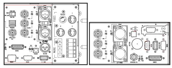
Connect the DB9 connector to the I<sup>2</sup>C BUS or SERVICE/RDS (depending on model) of /RDS-TEX2HE & /RDS-TEX3HE option to the two BNC ouputs named 19KHZ PILOT OUT (synchronization signal) and SCA1/RDS (RDS signal) always present in the back of the machine itself. If the connecting device is different, identify an equivalent.
