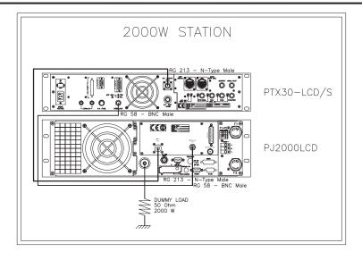
Figure 5.1: connections with amplifier
