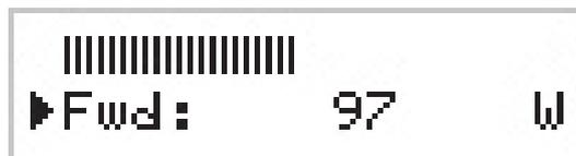
The lower line shows the instantaneous power reading (in this example 97W), while the bar indicates the set level. To increase the level, press the RIGHT/DOWN key, to decrease it press LEFT/UP. As the set level increases or decreases, the bar will become either longer or shorter to display the current setting. Once you have reached the desired level, press ENTER to confirm and exit the preset menu.
