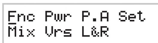
To enter one of the submenus, select the name (which will be underlined by a flashing cursor) with the LEFT or RIGHT keys and press ENTER.
