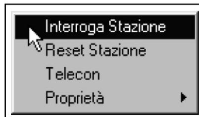
When selecting "Reset Station" you can make an attempt to reset the functioning conditions in case of alarm.
