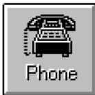
The "Phone" button enables to open the window showing the set-up of the telephone numbers saved in the memory of the SCM.
