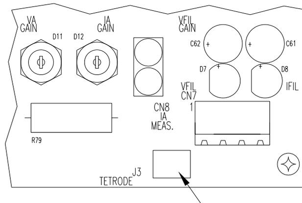
If the short-circuit is on J4 the card is been set for a triode amplifier.
