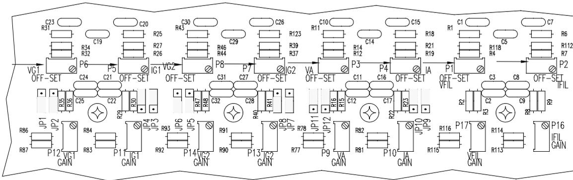
For reading the voltage values using always the multimeter with the negative connected to ground and the positive connected to relative test point in according to the value that you want calibrate.
