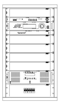
This version of the transmitter is tele-controllable and includes the RDS coder.
