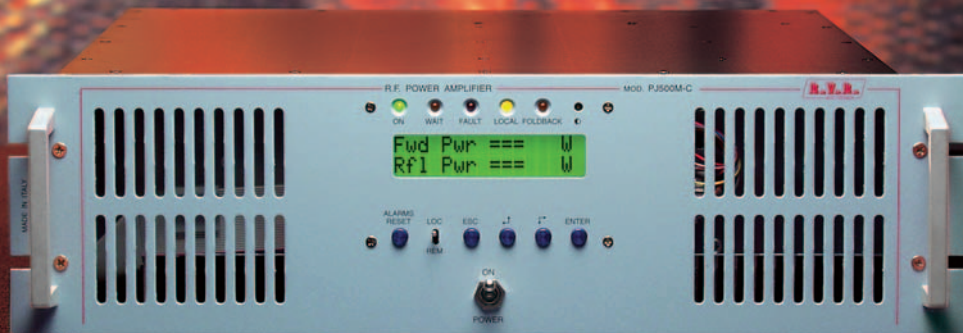
FM Mosfet Amplifier 87.5-108 MHz range
